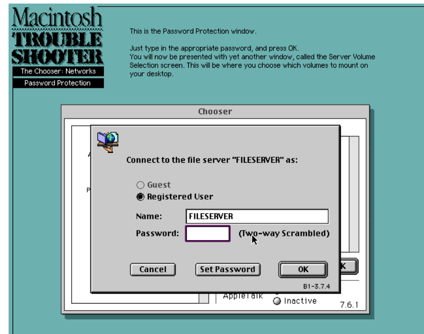
Picture 9.2 - Selecting a Fileserver - Type in the password, or be a guest.
